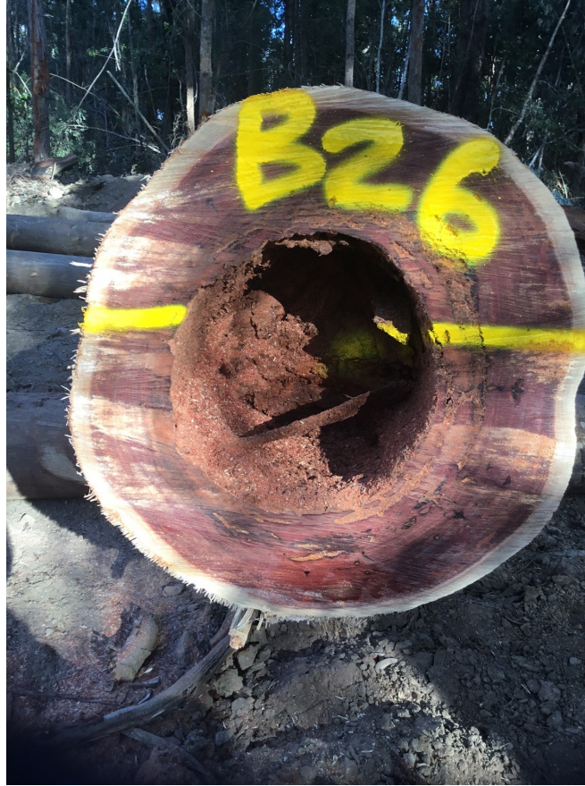
Figure 1: An example of a defective wood trunk.
